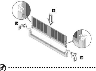
**Note:** The DDR2 DIMM sockets are slotted to ensure proper installation. If you insert a DDR2 DIMM but it does not fit easily
